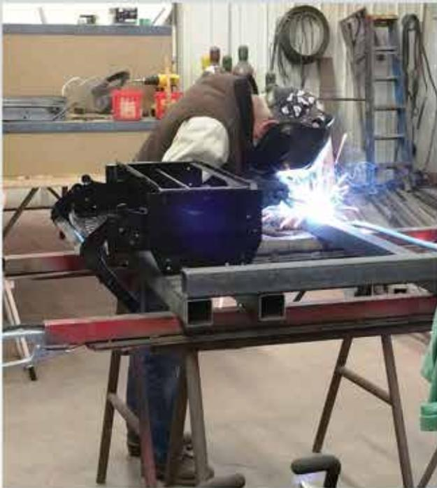
Terry Pierce of Belgian Hill Farm strikes an arc on the rear axle of the running gear. Note the retractable steps for easy access to the back of the wagon have already been attached. The front axle of the wagon will be the full fifth wheel gear Terry makes for all of his wagons.
